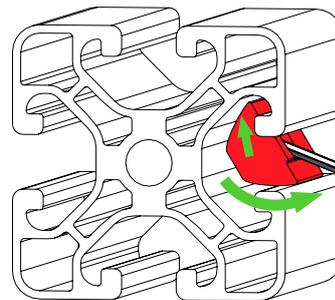
Move it a little back and forth while lifting up the slot nut and then turn it out.
