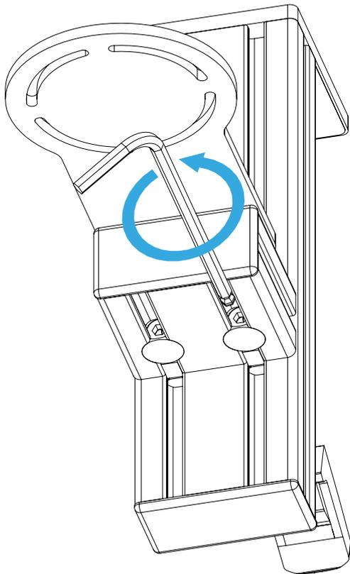
If you have a table mount already and want to mount the optional angle bracket then you have to unscrew the two universal connectors and remove the profile with the mounting plate.
