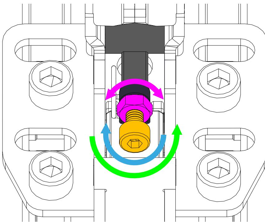
Loose the lock nut for adjustment.
