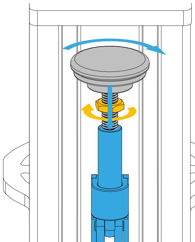
Turn pressure plate in and out to adjust the distance. A visible thread length of around 10mm (0.4") is recommended.
