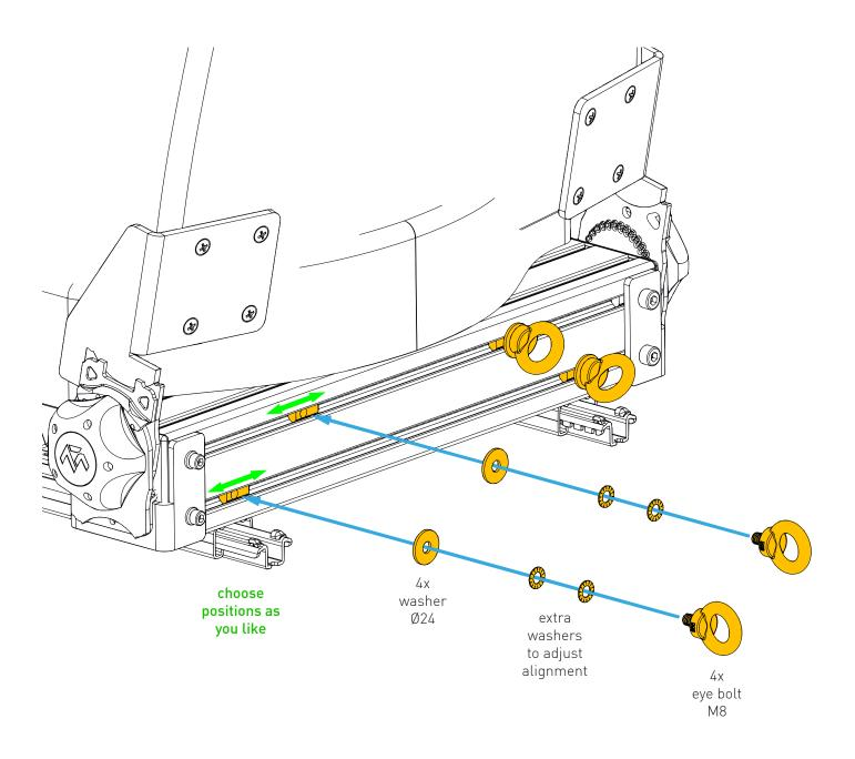
The alignment of the ring bolts after tightening is random (thread length given by engineer standard). To adjust the alignment extra washers can be used.
